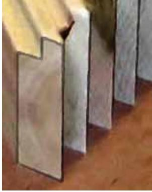
An inside edge lip is needed on all sides and ends so the table top can be dropped into place and glued. Cut this before you assemble the box. Also consider using a small roundover bit on the outside edge for splinter control and to reduce elbow, chin, and head dents later...
